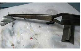
earpost wire at the right angle. The stand is just soldered up from scrap copper or nickel.
